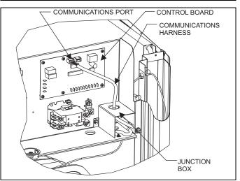
FIGURE 6: Communications Harness Connection
